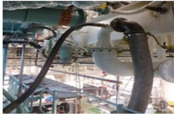
Main Engine L.O Flushing
