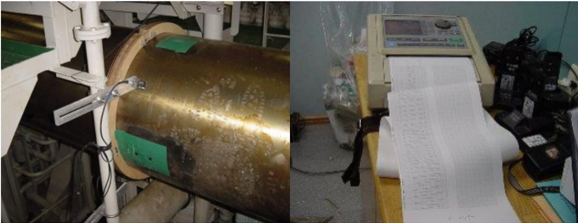
[Torsion Meter Calibration]
