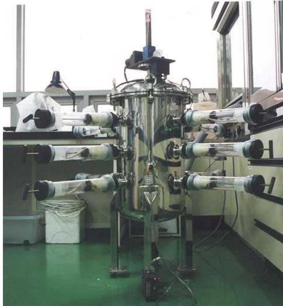
Figure 1. Nose only exposure chamber
