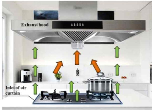
Fig. 5. Schematic diagram of push-push ventilation system (Zhou *et al.*, 2016).
