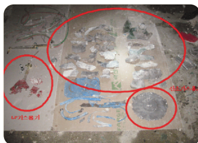
〈Recovered oxygen and LPG tanks and parts〉
