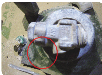
〈Inscription indicating the date of oxygen gas tank [(검) 00Y8-3]〉
